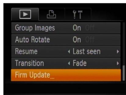
6. The firmware update confirmation screen appears, so select [OK], and then press the [FUNC./SET] button to start the firmware update.
